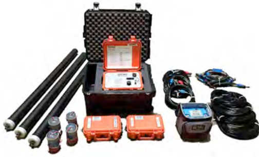
Figure 1: The main components of the array system: 1) KMS-820 digital acquisition system, 2) LEMI-120 low frequency magnetometer, 3) LEMI-701 electrodes, 4) KMS-831 sub-acquisition controller, 5) KMS-029 fluxgate magnetometer, 6) KMS-410 lithium ion battery, and 7) miscellaneous connection cable
